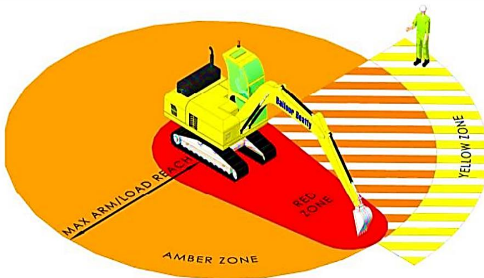
Gambar 18. Zona Keselamatan Excavator clamshell
