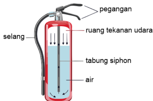
Gambar 6. 28 Bagian pada APAR Jenis Cairan (Air) (Sumber: https://image.shutterstock.com/image-vector/diagram-showing-inside-fire-extinguisher-260nw-1536503954.jpg )
